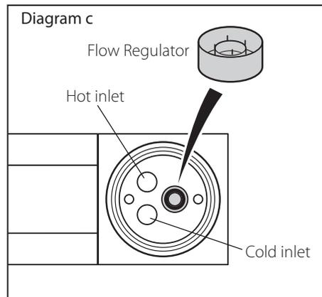
Replace the cartridge back into the mixer body making sure the 2 inlet holes are to the front.
