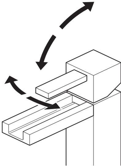
Moving the mixer lever upwards/downwards will increase/decrease the flow of water.
