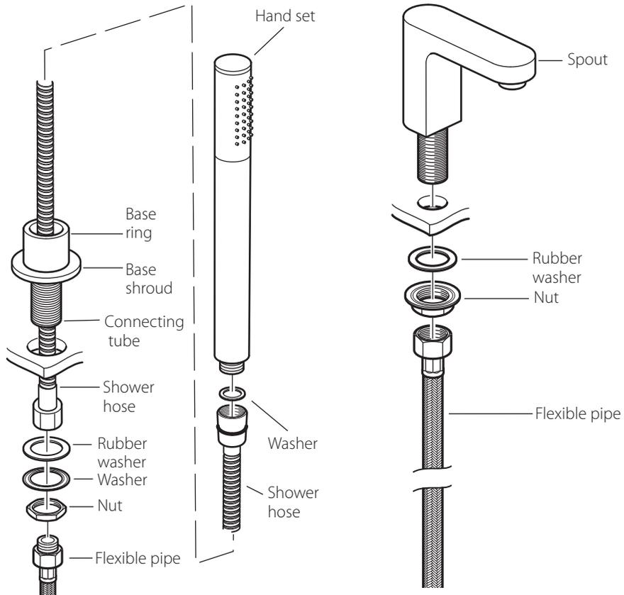
Remove the nut, washer and rubber washer from the connecting tube. Push the shower hose and connecting tube down through the hole, make sure the seal is in position in the bottom of the base shroud. From the underside slide on the rubber washer, metal washer and then the nut. Tighten the nut to clamp on the cover plate.
