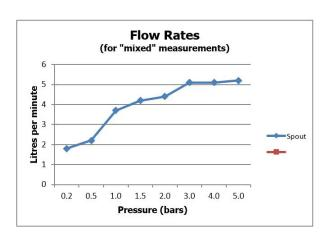
The flow rate displayed is calculated using ideal system conditions. This result should only be taken as an indication as the flow rate may vary depending on the specific in-situ configuration.
