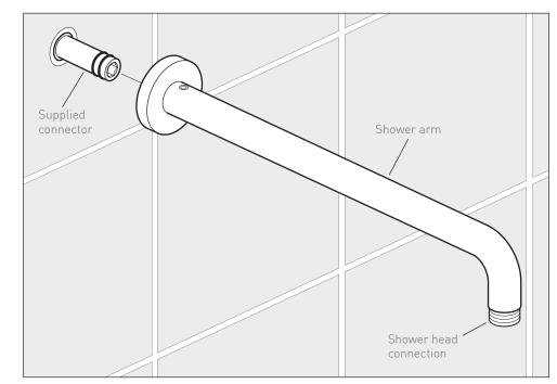
Carefully slide the shower arm onto the connector until it makes contact with the wall.
