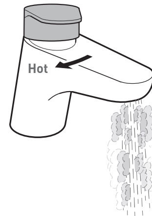
Moving the mixer lever from right to left will increase the water temperature.
