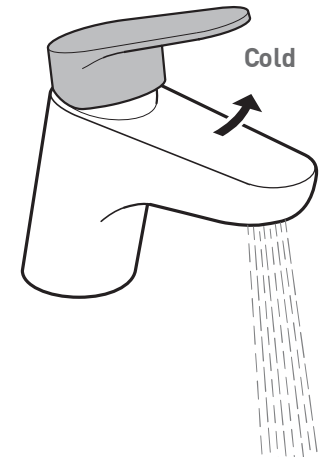
Moving the mixer lever from left to right will decrease the water temperature.
