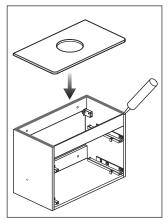
Apply a non-acidic silicone along the top edge of the unit and carefully position the countertop ensuring that it is flush with the sides of the vanity unit.
