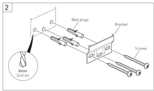
Drill Ø 8mm holes, insert the wall plugs and screw on the brackets. **NOTE:** If the vanity unit and/or basin are not fitted level this may pre-
