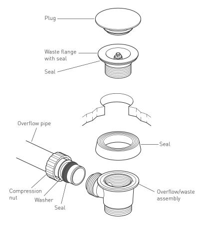
Push the seal onto the waste assembly
