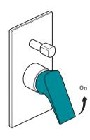
Pulling the mixer lever outwards will increase the flow of water.
