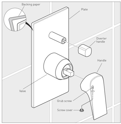
Remove the backing paper from the seal located on the back of the plate. Slide the plate over the valve, push onto the wall until it makes contact.
