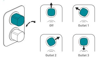
Turning the flow control handle to the required position increases the flow of water
