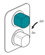
Turning the flow control handle in the direction of the arrow (anti-clockwise) increases the flow of water
