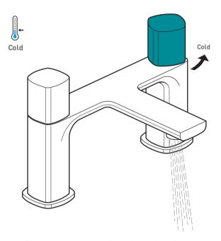
Turning the cold handle to the right will increase the flow of cold water.
