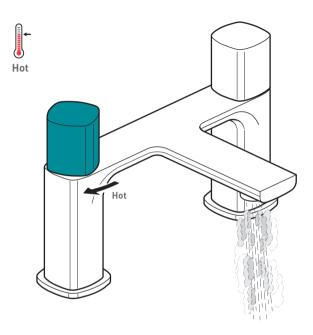
Turning the hot handle to the left will increase the flow of hot water.
