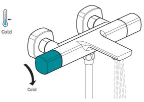
Turning the temperature control handle in the direction of the arrow decreases the water temperature
