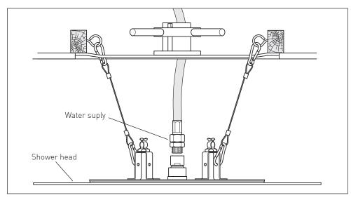
Using a flexible pipe connect the water supply to the shower head. Turn on flow and check for leaks.
