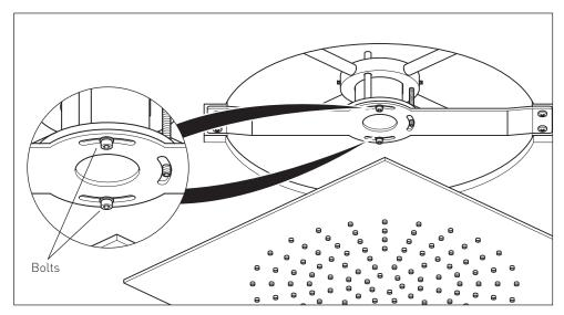
If fitting the square shower head and alignment is required with the edge of the room etc, there is the option for fine rotational adjustment once the bracket has been installed. Undo the 2 bolts underneath the bracket and rotate the arms to the desired location, then secure the bolts again.
