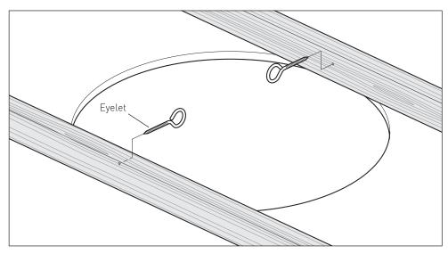
Securely screw the two eyelets into the ceiling joists/support.
