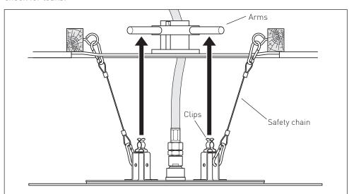
Align the clips directly below the arms, push the shower head until the clips snap into position.
