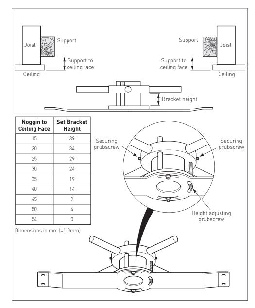
Measure the distance between the bottom surface of the support and the face of the ceiling, then use the reference table to determine what height to preset the bracket at. Adjust the height using the grub screw, then secure into position with the top 2 grub screws.
