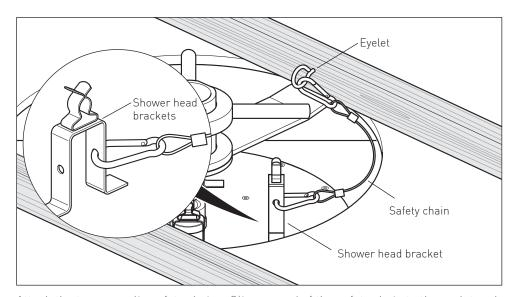
Attach the two easy clip safety chains. Clip one end of the safety chain to the eyelet and the other end into one of the holes on the shower head bracket. Repeat for the other side.
