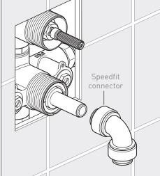
We recommend to push a speedfit connector (not supplied) over the drain, and place a bucket underneath. If a speedfit connector is not being used, carefully hold a bucket underneath the drain valve.
