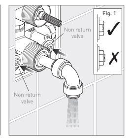
Turn on at the mains, open both non return valves and allow the debris and water to drain. When loosening the non return valve do not unscrew further than the face of the nut **(see Fig. 1).** After approximately two minutes of flushing the pipe work and product close both non return valves. Do not overtighten.
