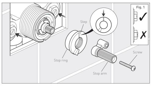
Push the stop ring onto the splines of the cartridge, making sure that the step on the stop ring is at 12 o'clock. Slide the stop arm on and secure in position with the screw. Open both non return valves.
