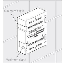
Finish the wall by tiling up to the mortar guard, keep the final finished wall surface between the min and max marks.
