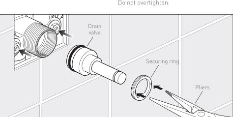
Close both non return valves. Remove the speedfit connector. Using a pair of long-nosed pliers unscrew the securing ring and remove. Pull the drain valve out from the body Installation
