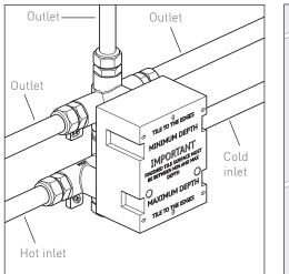
Connect hot supply to the lower left inlet of the valve and cold supply to the lower right inlet. Connect the open outlets to desired channels.
