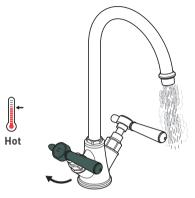
Turning the hot handle clockwise will increase the flow of hot water.
