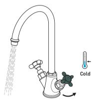
Turning the cold handle anti-clockwise will increase the flow of cold water.
