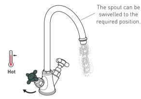
Turning the hot handle clockwise will increase the flow of hot water.
