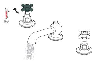
Turning the hot handle clockwise will increase the flow of hot water.
