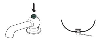
Push the waste control rod down to open the plug and empty the basin.
