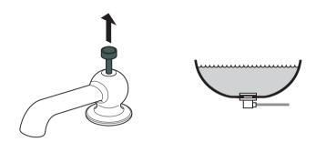
Pull the waste control rod up to close the plug and fill the basin.
