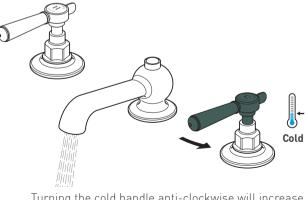
Turning the cold handle anti-clockwise will increase the flow of cold water.
