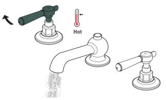
Turning the hot handle clockwise will increase the flow of hot water.
