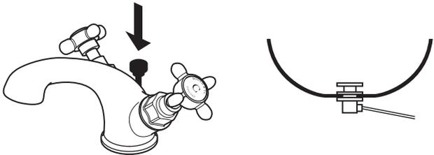
Push the waste control rod down to open the plug and empty the basin.
