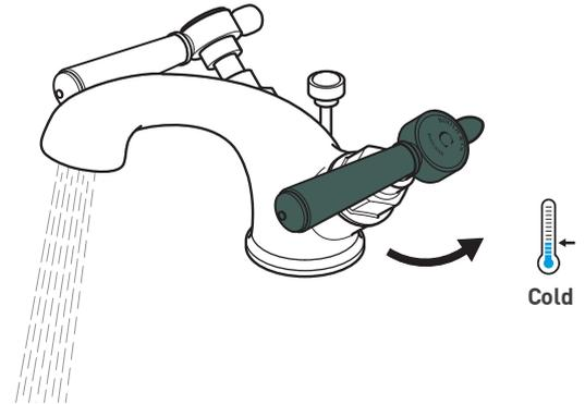
Turning the cold handle anti-clockwise will increase the flow of cold water.
