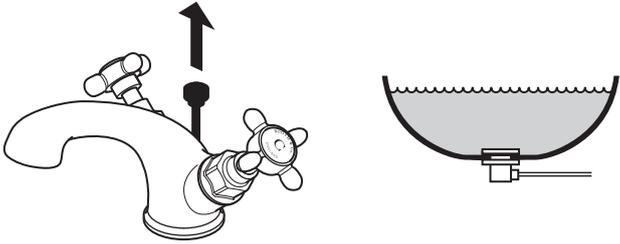
Pull the waste control rod up to close the plug and fill the basin.
