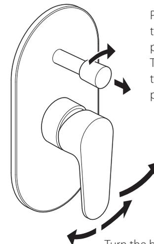
Pull the diverter handle and turn clockwise to lock into position. Turn clockwise again to release the diverter and go back to the primary outlet.
