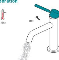
Moving the mixer lever to the left will increase the water temperature.
