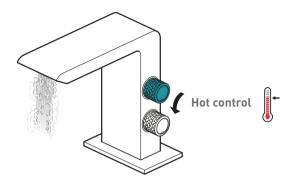
Turn the control forward to increase the flow of hot water
