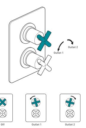
Turning the flow control handle in the direction of the arrow increases the flow of water
