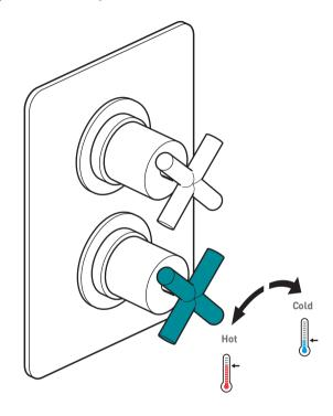
Turning the temperature control handle in the direction of the arrows increases/decreases the temperature
