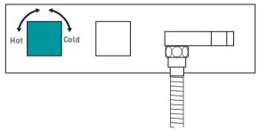
Turning the temperature control handle in the direction of the arrows increases/decreases the temperature
