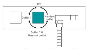
Turning the flow control in the direction of the arrows increases the flow of water to the outlets.
