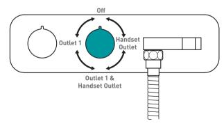
Turning the flow control in the direction of the arrows increases the flow of water to the outlets.
