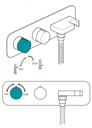
Turning the temperature control handle in the direction of the arrows increases/decreases the temperature
