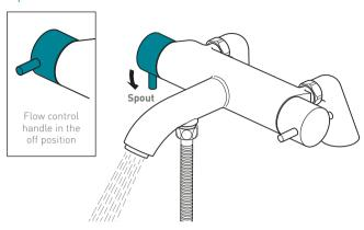
Turning the flow control handle in the direction of the arrow increases the flow of water to the spout
