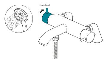
Turning the flow control handle in the direction of the arrow increases the flow of water to the handset
