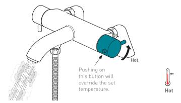
Turning the temperature control handle in the direction of the arrow increases the water temperature
