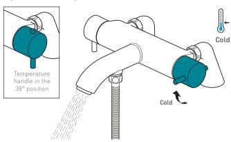
Turning the temperature control handle in the direction of the arrow decreases the water temperature
