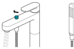
Turn clockwise again to release the diverter and go back to the primary outlet.
