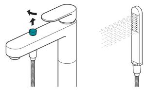
Pull up the diverter handle and turn clockwise to lock into position.
