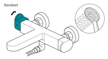
Turning the flow control handle in the direction of the arrow increases the flow of water to the handset
