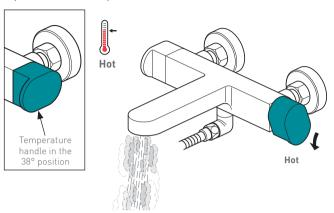
Turning the temperature control handle in the direction of the arrow increases the water temperature
