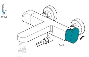
Turning the temperature control handle in the direction of the arrow decreases the water temperature
