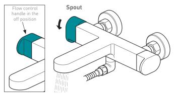
Turning the flow control handle in the direction of the arrow increases the flow of water to the spout
