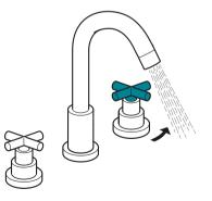
Turning the cold tap anti-clockwise increases the flow of cold water
