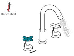
Turning the hot tap clockwise increases the flow of hot water
