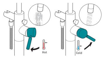
Moving the mixer lever to the left will increase the water temperature.
