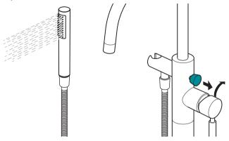
Pull out the diverter handle and turn clockwise to lock into position.
