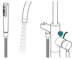
Turn clockwise again to release the diverter and go back to the primary outlet.
