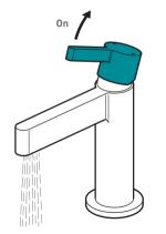
Lifting the mixer lever upwards will increase the flow of water.
