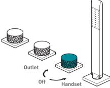
Turning the diverter handle clockwise activates the flow of water progressively to the desired outlet. Turning the diverter anti-clockwise activates the flow of water progressively to the handset.
