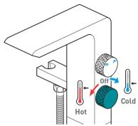
Turning the temperature control handle in the direction of the arrows increases/decreases the temperature
