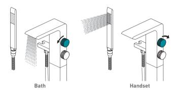
Turning the diverter handle anti-clockwise activates the flow of water progressively to the bath.
