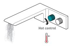
Turn the control clockwise to increase the flow of hot water
