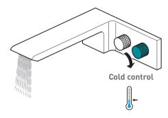
Turn the control clockwise to increase the flow of cold water
