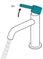
Lifting the mixer lever upwards will increase the flow of water.
