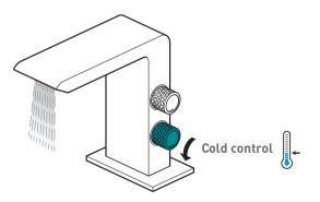
Turn the control forward to increase the flow of cold water
