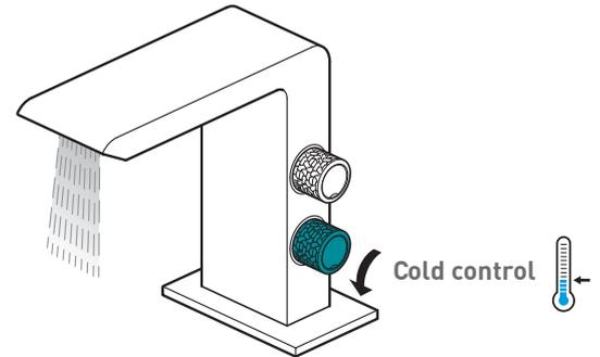
Turn the control forward to increase the flow of cold water
