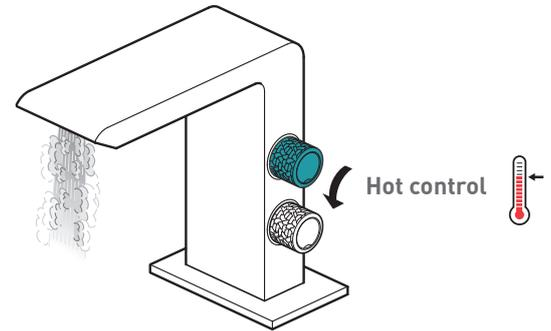
Turn the control forward to increase the flow of hot water
