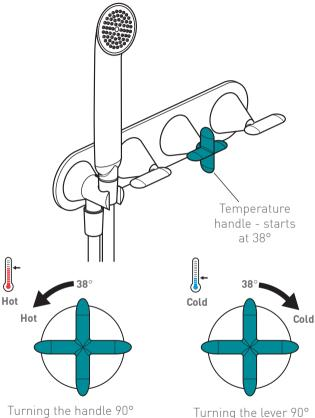
Turning the handle 90° anti-clockwise will increase the temperature. up to a maximum of 46°
