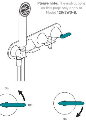
Turning the handle 90° anticlockwise will progressively increase the flow of water to outlet 2.
