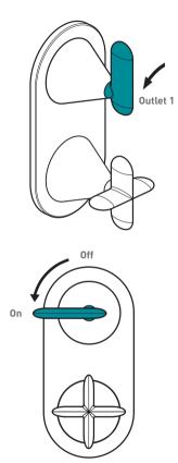
Turning the flow control handle in the direction of the arrow increases the flow of water to the outlet.
