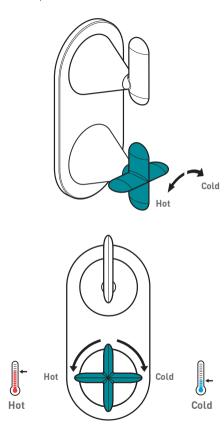
Turning the temperature control handle in the direction of the arrows increases/decreases the temperature
