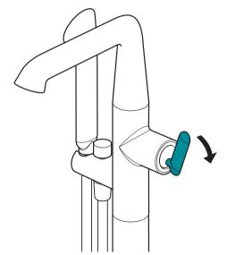
Pulling the mixer lever outwards will increase the flow of cold water.
