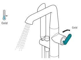
Pushing the mixer lever backwards will increase the flow of cold water.
