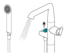
Pull up the diverter handle to change flow to handset.
