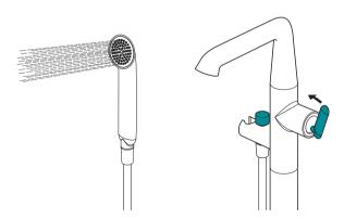
Handset will automatically shut off when the flow handle is turned off.
