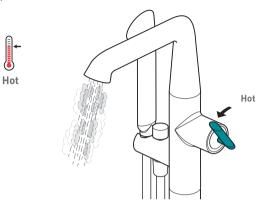
Pulling the mixer lever forwards will increase the flow of hot water.
