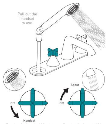
Turning the handle 90° anticlockwise will progressively increase the flow of water to the handset (Outlet 2).
