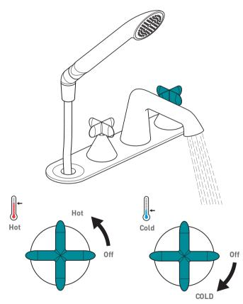
Turning the handle 90° anti-clockwise will increase the temperature.
