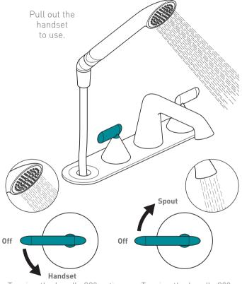
Turning the handle 90° anticlockwise will progressively increase the flow of water to the handset (Outlet 2). Turning the handle 90° clockwise will progressively increase the flow of water to the spout (Outlet 1)
