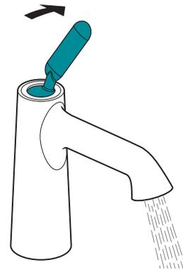
Rotating the handle to the right changes flow and temperature simultaneously.
