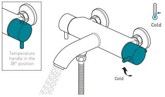
Turning the temperature control handle in the direction of the arrow decreases the water temperature
