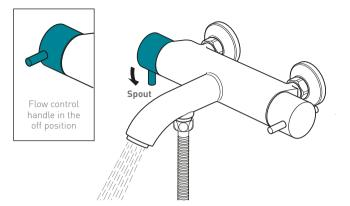
Turning the flow control handle in the direction of the arrow increases the flow of water to the spout
