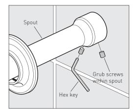
Slide the spout along until it makes contact with the wall.
