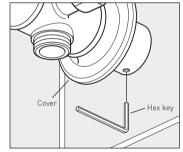
Slide the cover along until it makes contact with the wall.
