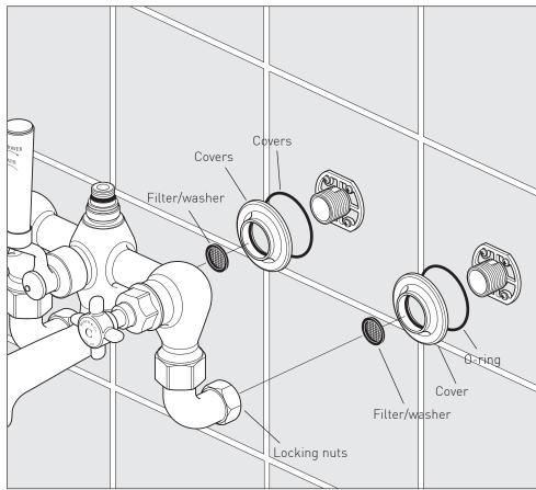
Slide the covers over each connecter. Place a rubber filter/washer in each of the locking nuts on the valve and screw onto the connecters.
