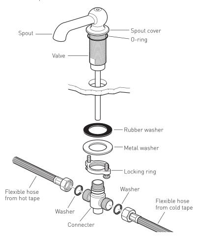
Make sure the 0-ring is in place in the underside of the spout cover.
