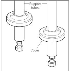
Slide the foot plate over the support tube pipe and into the support tube.
