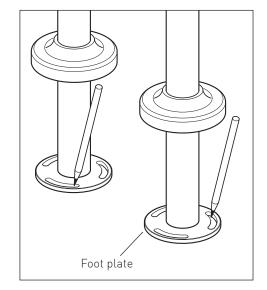
Drill the 6 holes to the required depth and diameter to suit your fixings and floor.
