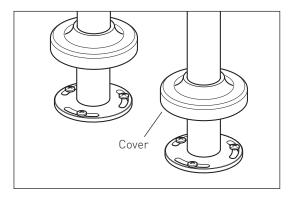
Carefully screw the handset holder onto the valve. Make sure that it is in the correct position before tightening.
