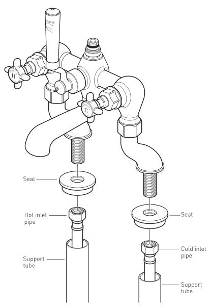
Slide both seats onto the mixer connections.
