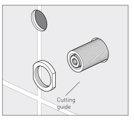
Using a hacksaw along the side of the cutting guide cut through both the handle extension and spline extension. Remove the cutting guide clean up any burrs and remove any debris. Repeat for the other side.
