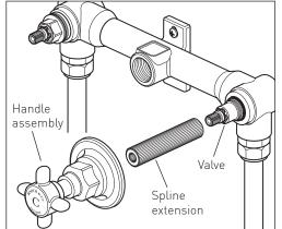
Using light force only turn the handle clockwise until you feel a noticeable resistance when the base of valve touches down on the body of the tap. Turn the handle so the valve is in the closed position, then remove the handle.
