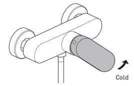
Moving the mixer lever from right to left will increase the water temperature.
